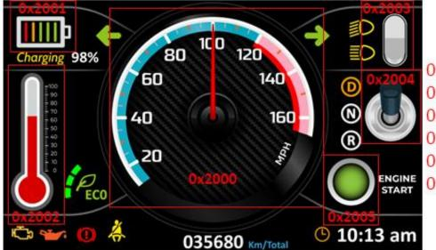
0x2000 Gauge 0x2001 Battery 0x2002 Temperature 0x2003 Toggle Button 0x2004 Toggle Button 0x2005 Indicator
